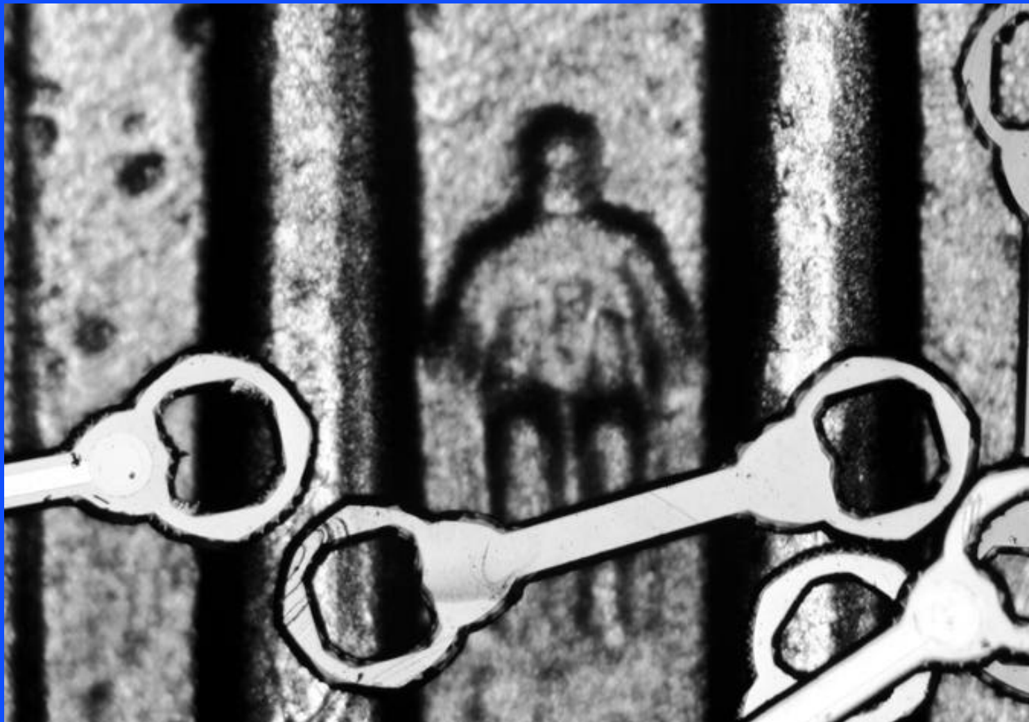
Implantable strain gauges on a penny.
